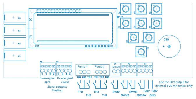
If the thermostatic switches TH2 and TH4 are not necessary, bridges have to be inserted on those contact points. The thermostatic switches TH1 and TH3 can be deactivated via the menu therm. malfunction.
